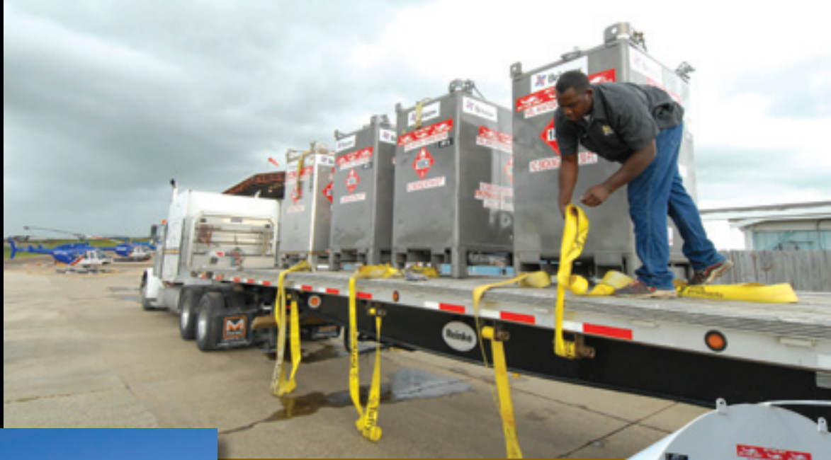
Driver straps down tote tanks on flatbed trailer
