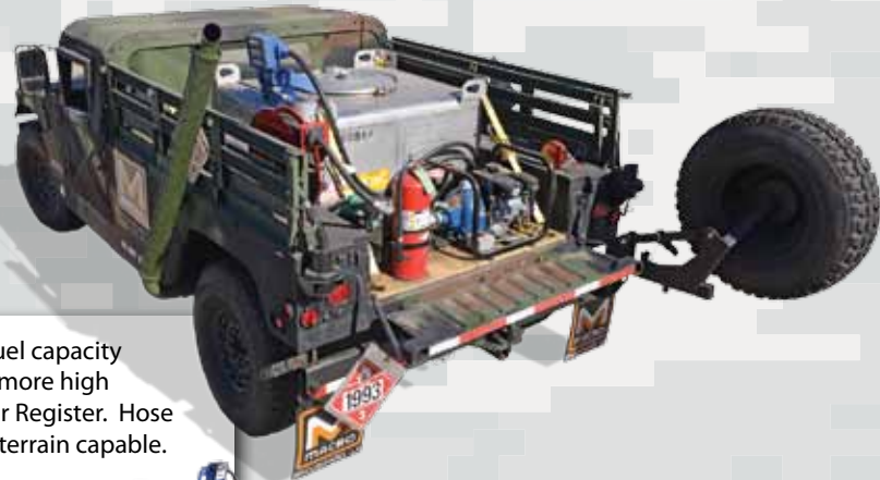
Military Style Utility Trailer with 350 gallon tank. High volume pump and backup 12 Volt Pump (Optional solar panel).
