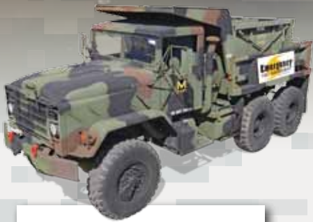
Military Dump Truck with one fuel tank (900 gallon capacity). High volume pumping system. High water / all terrain capable.
