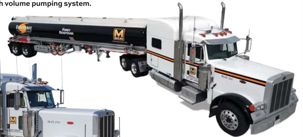
Mobile fueling trailer. 8,500 gallon capacity. Multi-compartments. Dedicated pumping system, meters, hoses and nozzles specifically designed for refueling vehicles.
